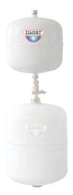
According to our experience and the reviewing of different international regulations on solar energy an additional tank is recommended when the fluid volume between the collector and the expansion vessel is approx 50% or less than the 'wet' side volume (between the expanded diaphragm and the vessel inlet). This approach is covered by the European Directive VDI 6002.
