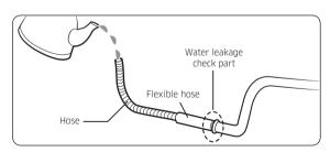
**b** After pouring some water, reassemble the rubber cap on the connection part of a flexible hose of the indoor unit and firmly tighten it with a band to prevent leakage.
