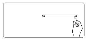
3 Rotate the paper compass on its pivot point to draw a line on the ceiling.
