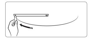
4 Rotate the paper compass diametrically to draw a circle on the ceiling.
