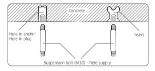
**4** Install the suspension bolts, depending on the ceiling type.
