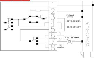
Link 4 & 5 for fan continuous mode, 3 & 5 for fan thermostatic mode.
