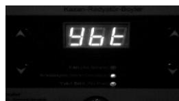
Fuel-Out Set Value Option Menu: When you push and hold FAN DOWN button for ten seconds there will be Y and SET value on screen like a pictur down below, it can be change by using FAN DOWN and FAN UP buttons. When you stop holding buttons , set value will be recorded automatically and screen return to the normal menu. When calculated heat increase over the set value and decrease down set fuel-out value , system give an warning like upside picture.
