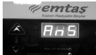
When there is a problem about heat system calculator, system give an mistake code and voice alert then start the circulation pump by turn off the fan.
