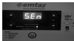
Fuel - Out Warning: System does not give an fuel-out warning without calculate the pump set value at least one time after the heating boiler open. Boiler give an YBT(fuel-out) warning when it see the calculated Fuel-Out set value.
