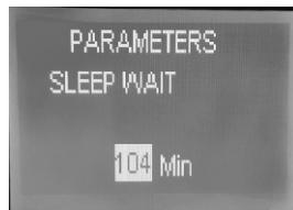
STAND BY: Push the MENU button after the stand by time set, stand by mode is going to open. This menu shows the supply period time in the heating boiler. For example, if you enter the normal supply time is 7 seconds, stand by supply time is 20 minutes, the heating boiler will do 7 seconds supply in every 20 minutes.
